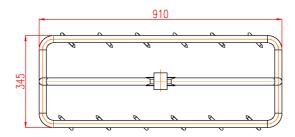
The kit for offal is used for offal hanging and transport on flat-bar and round-bar railways at beef and pork slaughters. The frame is welded from stainless steel tubes. There are hooks welded to the frame – for hanging the offal. The whole kit is pivoted on the hook for flat-bar railway.
